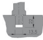
Tool slot to suit for NS V and NS VI adaption
