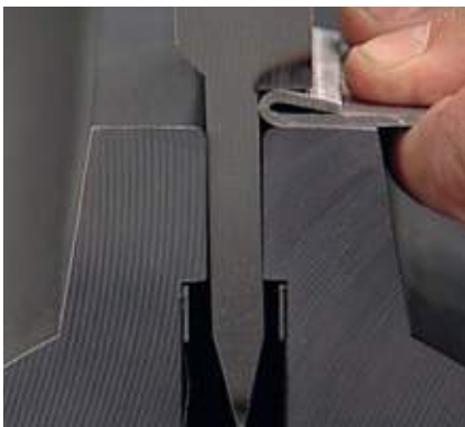
Pre-bend and flattening in the same tool.
